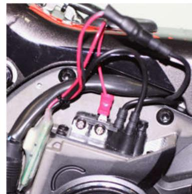
④ Place the MSO in a proper position and optionally, fasten the wiring using the electrical ties. Re-attach the plastic cover and the bike is ready to go.
