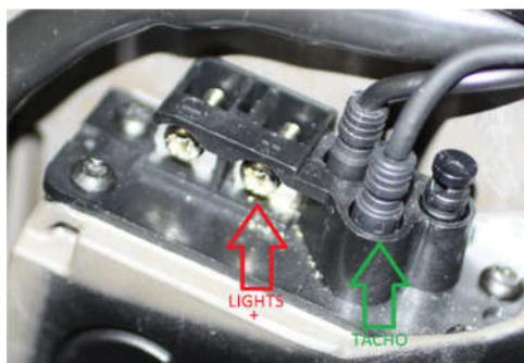
③ Connect the speed sensor to the MSO unit and the MSO unit to the motor unit using corresponding connectors. Connect red power cable to positive light clamp. Tighten the screw of the clamp.
