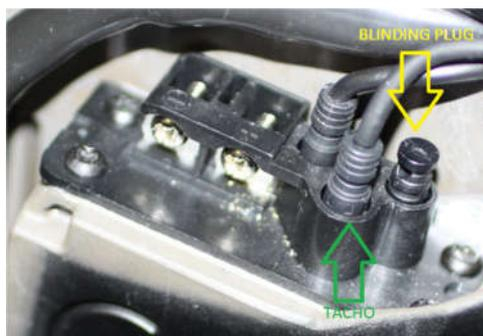
③ Take care about wiring in this step. A mistake can cause serious damage to the MSO or to the bike. Connect **red marked** MSO cable instead of the blinding plug. Connect other two MSO cables between the speed sensor to and the motor unit using corresponding connectors.
