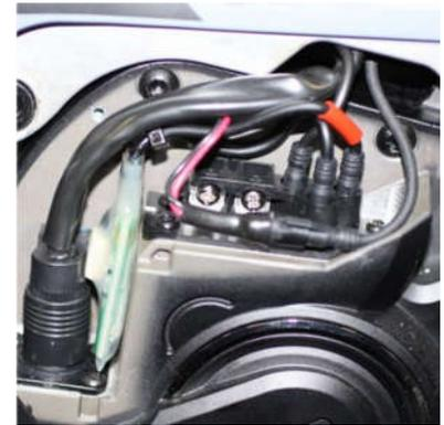
④ Place the MSO in a proper position and optionally, fasten the wiring using the electrical ties. Re-attach the plastic cover and the bike is ready to go.
